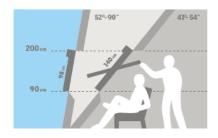
Top-operated centre-pivot roof windows make it possible to place furniture directly below the window without obstructing operation of the window.
